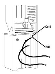
STEP 3. Attach the hose with the blue coupling to the cold water (top) inlet valve. Screw on coupling by hand. Make an additional two-thirds turn with pliers to tighten coupling. DO NOT OVER-TIGHTEN; this could damage valves.
